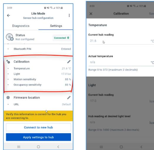
Figure 4. Calibration Tool
