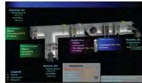
Air Handling Unit ORCAView
