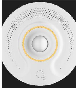
If there is an error, the light ring will flash red 3 times. Check your file location, name, and connection. The sensor hub will attempt the upgrade a maximum of 3 times.
