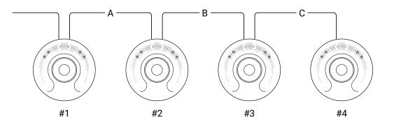
The hubs have a bypass switch that allows them to continue relaying data after losing power. In a power failure scenario, the maximum cable length is reduced by 15 m (50 ft) for each bypassed hub.
